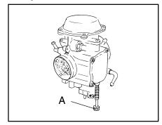
3. Adjust the carburetor idle screw (A) in or out until the desired idle RPM is reached. Turning the screw in (clockwise) will raise RPM. Turning the screw out (counterclockwise) will lower RPM.
